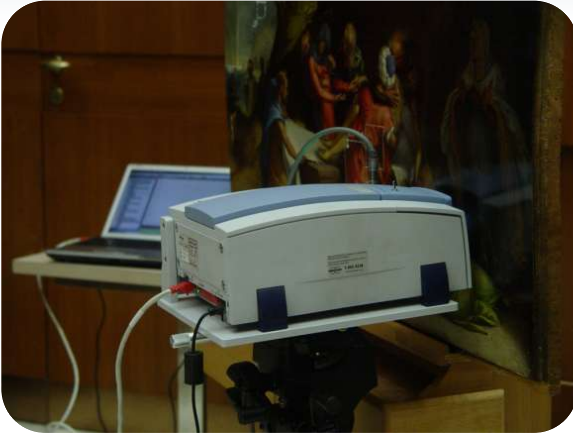
Standard tripod with geared head and adaption baseplate with focus position adjustment
